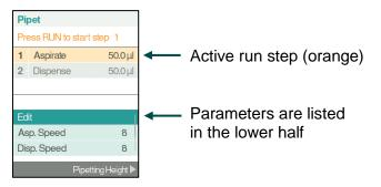
Insert the GripTips into the liquid to be transferred. Press and release **RUN** to aspirate the volume selected in the first step.
